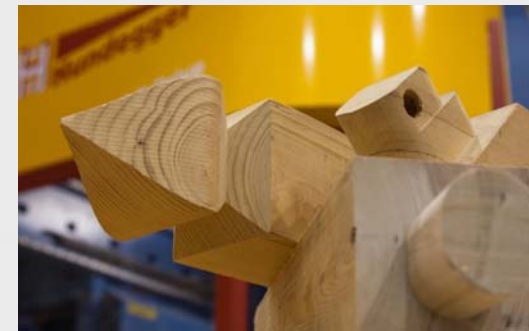
Timber Joinery created with Hundegger® Robot-Drive
